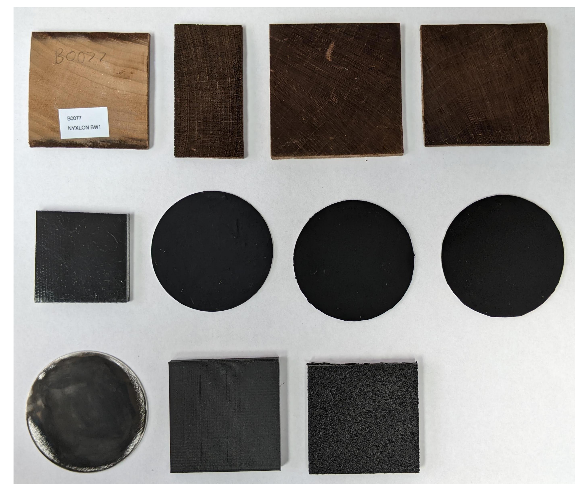
Figure 4. (Row 1, L to R) B0077 Nyxlon back side (to show original color), B0099 Nyxlon J, B0100 Nyxlon L, B0101 Nyxlon 3. (Row 2, L to R) B0095 Garolite G-10/FR4, B0096 Black 3.0, B0097 Fineshut SP, B0098 Fineshut KIWAMI (Row 3, L to R) B0102 Birchwood Casey Aluminum Black, B0106 Black PLA Default print, B0107 Black PLA "Fuzzy" print.
